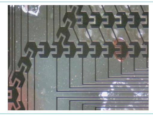
Real time transport of 100 picolitre droplets Velocity 1 mm / second
